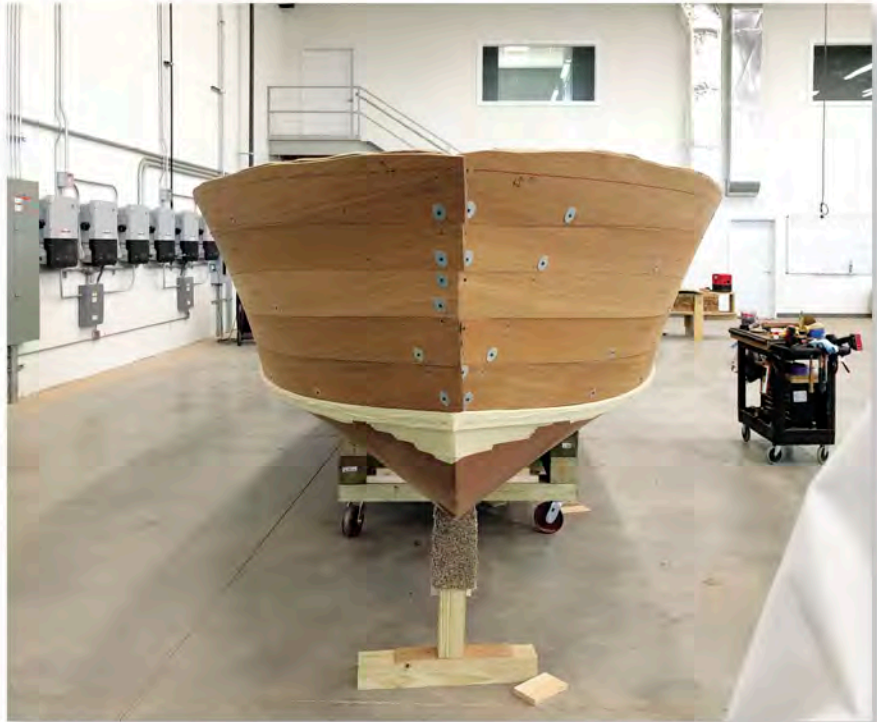
The Grand Craft 26' Burnham shows its book-matched planking and a convex bottom that Steve Northius calls the Gage-Hacker bottom. Wall-mounted power units, at left, convert the power from the roof's solar panels from DC current to AC current.
