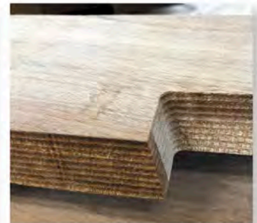
The bottom of the Burham 26-footer has three diagonal layers and hull sides have two diagonal layers and one horizontal.
