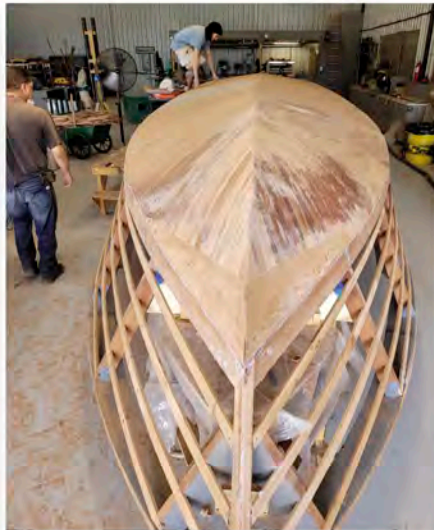
The bottom of the Burham 26-footer has three diagonal layers and hull sides have two diagonal layers and one horizontal.
