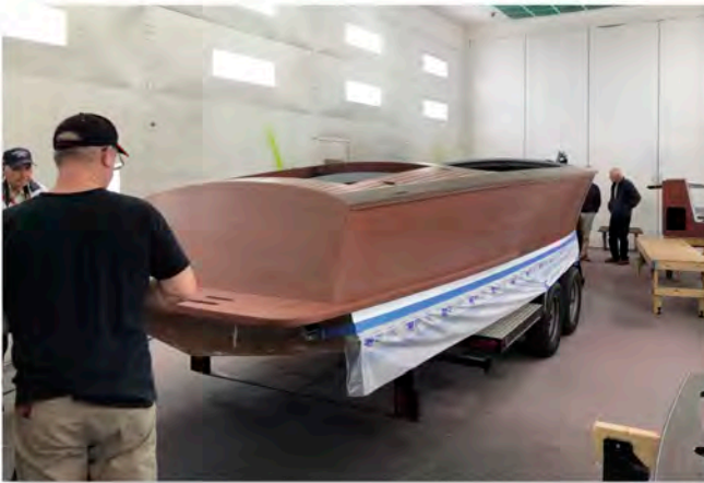
The final varnish coat is sprayed on in the neighboring professionally constructed spray booth that meets all the myriad stringent regulations.
