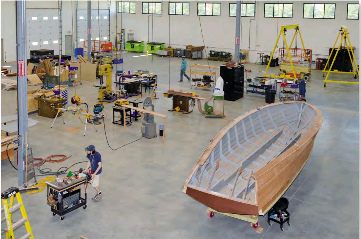
The shop floor is arranged for building twenty boats a year by progressing through various stations around the perimeter.
