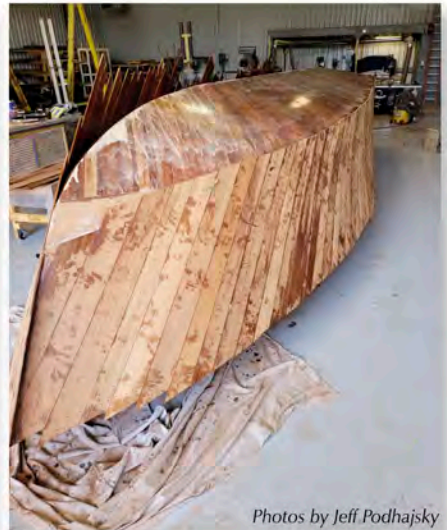
The bottom of the Burham 26-footer has three diagonal layers and hull sides have two diagonal layers and one horizontal.
