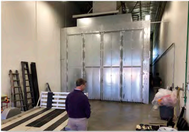
The final varnish coat is sprayed on in the neighboring professionally constructed spray booth that meets all the myriad stringent regulations.
